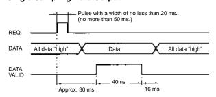
Approximately 30 ms after the REQ signal rises, a sample is taken and the DATA VALID signal is output. Read the data when the DATA VALID signal is ON.
